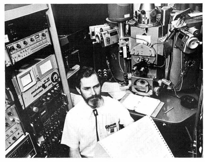
COMPUTER, BILL CHAMBERS with tab run of data, and electron microprobe (left to right). A focused beam of electrons in the probe strikes sample in the tank (to the right of Bill's shoulder). Three detectors in the tank are coupled, through amplifiers and analyzers, to a set of counters controlled by the computer (left). Stepping motors mounted on the tank can position the detectors or the sample itself — they're computer controlled too.
